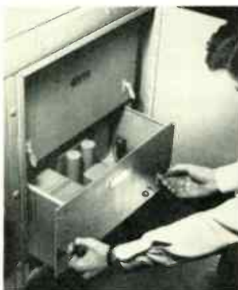
Alden Universal Scanner showing ease of removal and replacement of electronic chassis.
