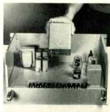
Regulator chassis, indicating ease of replacement or substitution of subcarrier oscillator through plug-in construction.
