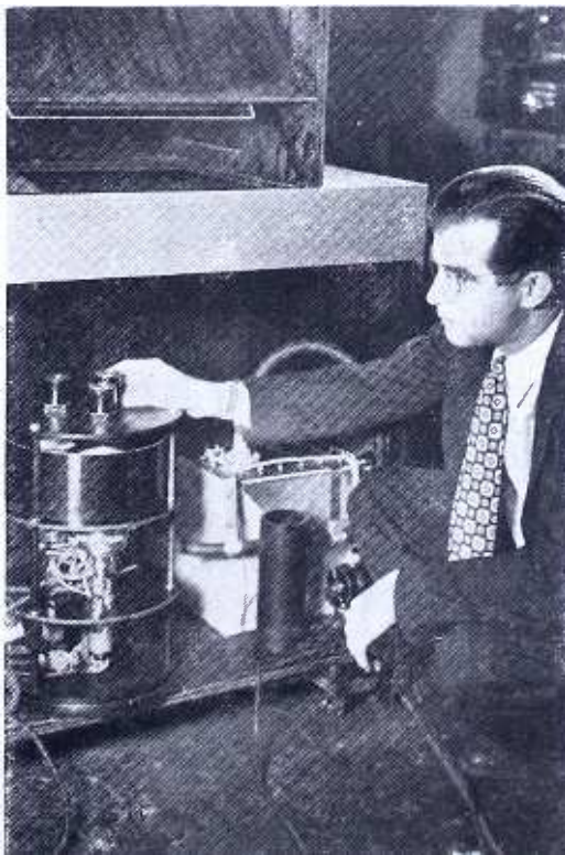
AT RECEIVER, RED, BLUE AND GREEN TUBES SUPPLY COLORS SIMULTANEOUSLY BELOW: RCA COLOR PROJECTION SYSTEM
