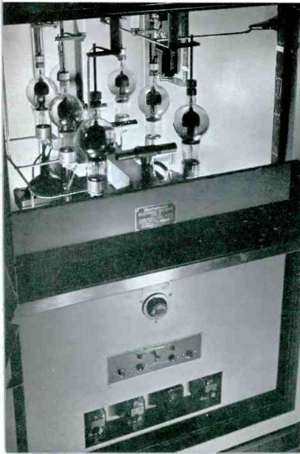
FIG. 7. THE RECTIFIER PORTION OF THE HIGH-VOLTAGE POWER SUPPLY TO THE FINAL POWER AMPLIFIER STAGE
