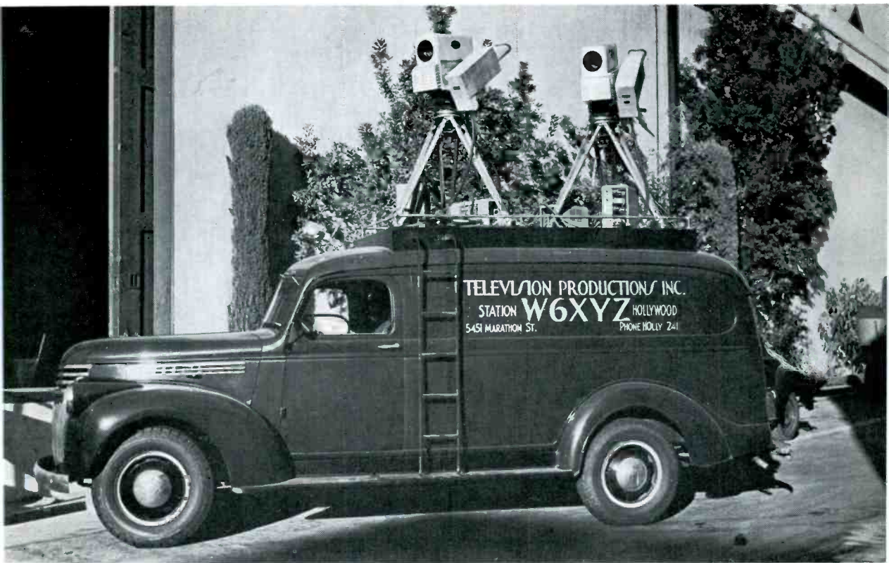
COMPLETE 2-CAMERA EQUIPMENT IS CARRIED IN THIS 3/4-TON TRUCK. THE CAMERAS CAN BE OPERATED FROM THE ROOF PLATFORM, OR SET DOWN ON THE GROUND
