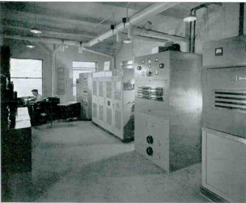
FIG. 1. THE 50-KW. TRANSMITTER, LOCATED ON THE 45TH FLOOR OF THE FIELD BUILDING. FIG. 2, CENTER, TRANSCRIPTION TURNTABLES AND
