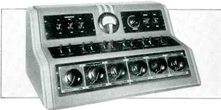
FIG. 1. ALL THE STUDIO EQUIPMENT CONTROLS ARE LOCALIZED IN THIS CONTROL ROOM CONSOLE. THE ASSOCIATED AMPLIFIERS AND RELAYS ARE MOUNTED IN A SEPARATE RACK
