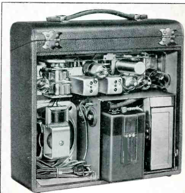
FIG. 2. REAR VIEW, WITH BATTERY COMPARTMENT COVER REMOVED. NOTE ARRANGEMENT OF RECTIFIERS, BATTERY, AND B VIBRATOR
