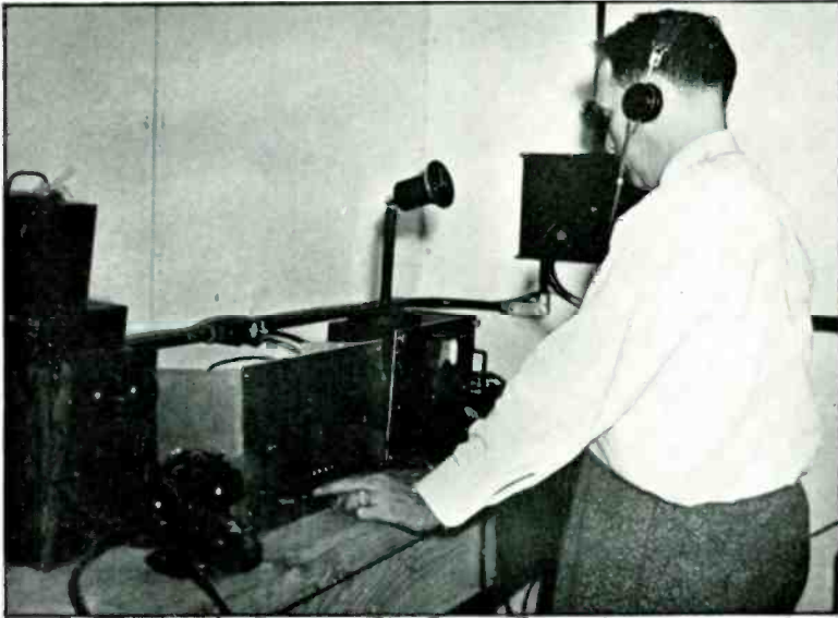
FIG. 9. SOUND CONTROL AT FRANKLIN FIELD HAS 4-POSITION MIXING AMPLIFIER AND COMPLEX ORDER SYSTEM CONNECTED WITH A TOTAL OF 5 TELEVISION CAMERAS
