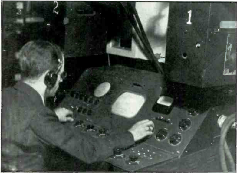
FIG. 5. PHILCO STUDIOS USE TWO TELEVISION CAMERAS FOR TRANSMITTING FULL-LENGTH MOVIES. THE MONITORING CONSOLE IS LOCATED BETWEEN THE CAMERAS
