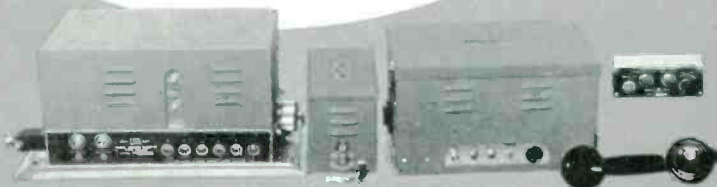
FMTR MOBILE ASSEMBLY Type 25 UFM 25/30 watt transmitter Type 11 UF receiver and power supply
