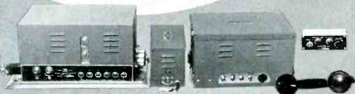
FMTR MOBILE ASSEMBLY Type 25 UFM 25/30 watt transmitter Type II UF receiver and power supply
