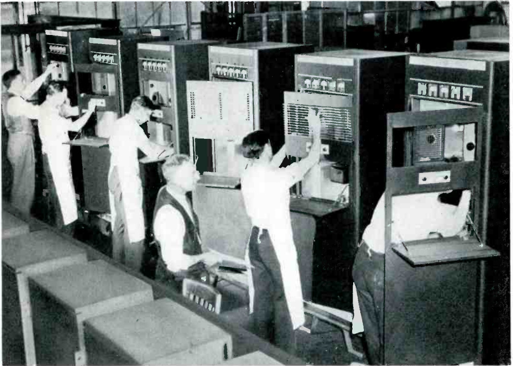
FIG. 6. ASSEMBLY LINE OF 1 KW. FM TRANSMITTERS AT GENERAL ELECTRIC'S SCHENECTADY PLANT. AMPLIFIER UNITS CAN BE ADDED TO INCREASE THE OUTPUT TO THE ANTENNA, IF NECESSARY
