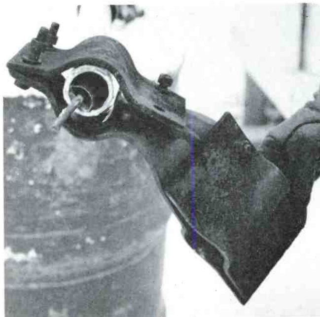
FIG. 8. FORCE OF STORM WAS ENOUGH TO BEND DIPOLE AND WARP CLAMP
