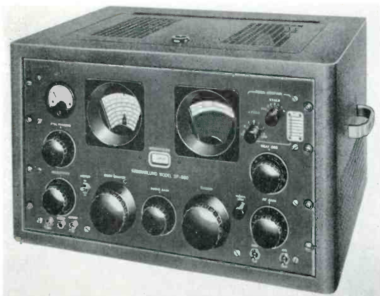
FIG. 1. SP-600JX RECEIVER IN TABLE-MODEL CABINET. SET CAN BE RACK-MOUNTED ALSO. FIG. 2. CHASSIS WITH SECTION COVER PLATES IN PLACE
