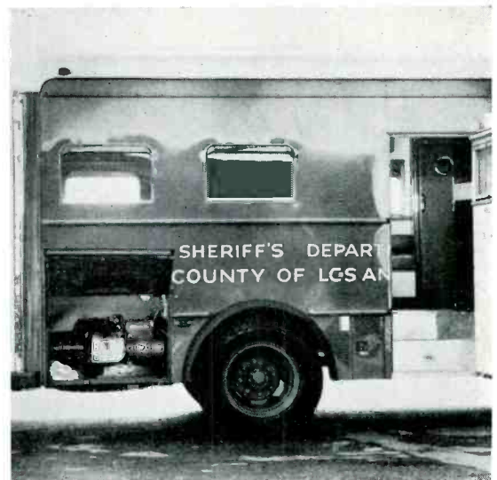
FIG. 9, LEFT: RADIO OPERATOR'S POSITION IS DIRECTLY BEHIND THE DRIVER. THIS VIEW, TAKEN FROM THE GALLEY, SHOWS THE ELECTRIC STOVE AND SINK. FIG. 10, ABOVE: COMPARTMENTS ON EACH SIDE AT THE REAR HOUSE THE 3-KW. ONAN ENGINE-DRIVEN GENERATORS
