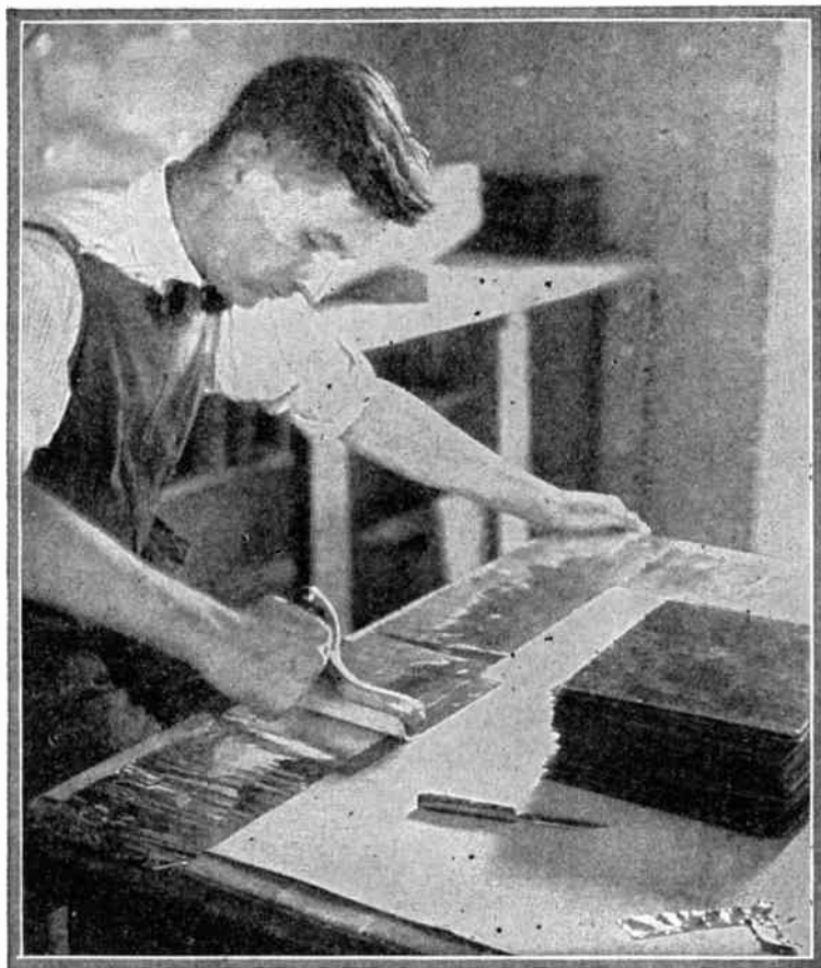
Fig. 1. Rolling out the wrinkles and creases in the tinfoil. If no photographer's roller is available, a bottle will do
