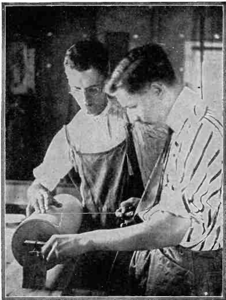
Fig. 3. Starting the winding. Note how the wire is guided
