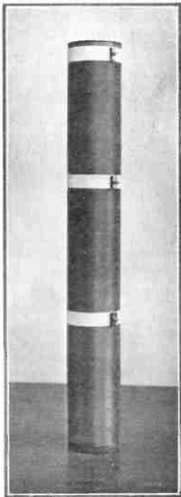
Fig. 1. One of the loading coils. Two coils are to be wound. Each consists of a single layer of wire on a cardboard cylinder
