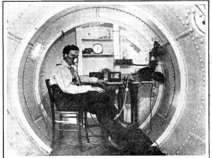
Interesting apparatus in the aero dynamic laboratory at St. Cyr, France. Car for testing propellers shown at left; caisson for testing pilot's ability to function normally in rarefied atmosphere shown at right
