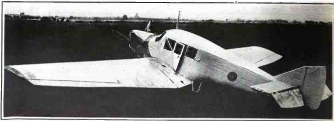
View of the JLo all metal internally trussed monoplane, an aircraft of German design and development that is recognized as the most efficient and economically operated airplane type yet built for commercial use
