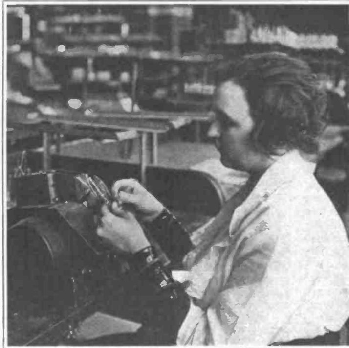
Winding the tungsten wire into incandescent lamp filament coils
