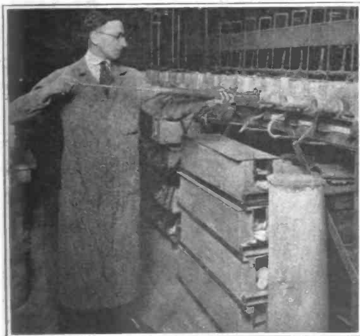
The operation of putting red hot tungsten bar through one of the many swagers whose revolving hammers chatter on all sides of the bar reducing it to smaller and smaller diameter is shown at the right
