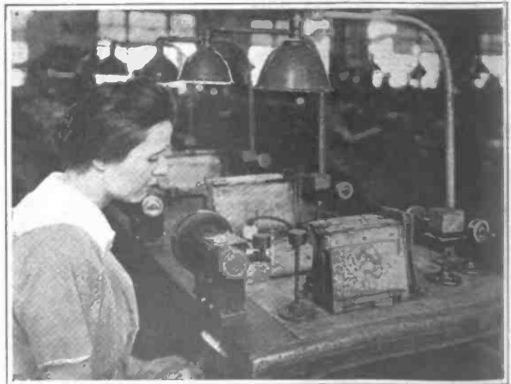
Drawing tungsten down to finest proportions, about four ten-thousandths of an inch is one-sixteenth of the size of fine human hair. It is used as filament in smallest "bug" lamps. The thread of tungsten passes through lubricant, then through gas furnace which has a diamond die at its end nearest the operator
