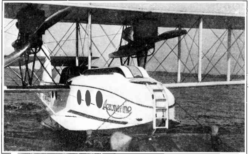
View of Aeromarine air yacht hull, showing cabin and location of power plants
