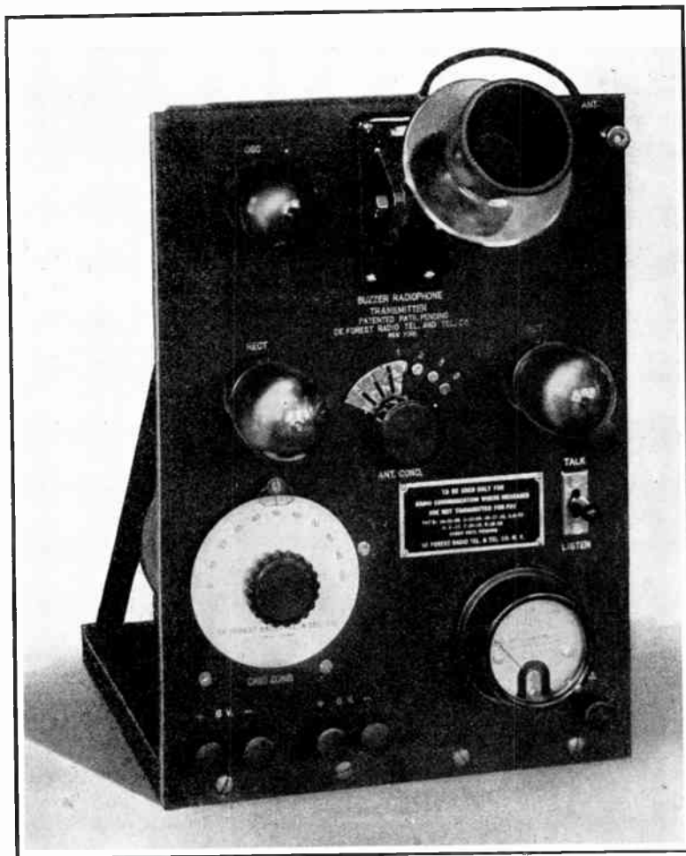
No motor-generators or high potential batteries are needed to operate this set
