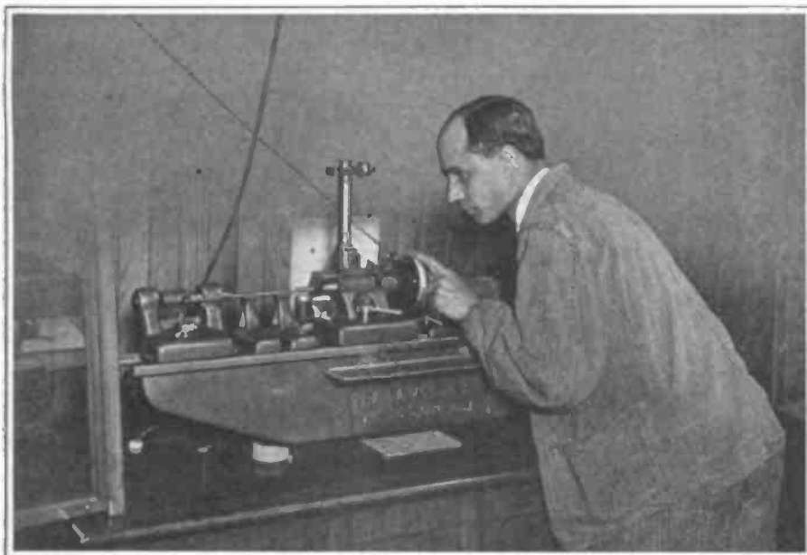
Precision measuring machine will measure to one-hundredth part of a thousandth of an inch
