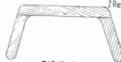
FIG. 1B-B A RECENTLY DEVELOPED FORM OF CABANE STRUT Section shown at Fig. T
