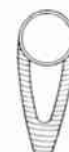
FIG. 1Q SPINDLED STRUTS With Balsa or Spruce fairing bound on with tape or linen.
