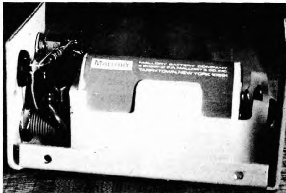
Fig. 3. The compact construction of the calibrator is seen here. We wired all components to the terminals of the banana jacks first, and then bolted in the battery holder to the bottom of the chassis to allow working room for assembly. You may choose to utilize either perboard or even a printed circuit board for your model. This will allow you to mount it directly inside the cabinet of whatever test instrument you wish to calibrate. With this method you can always have a reliable source of instrument calibration with you, no matter where you might happen to be doing your repair or field operations.
