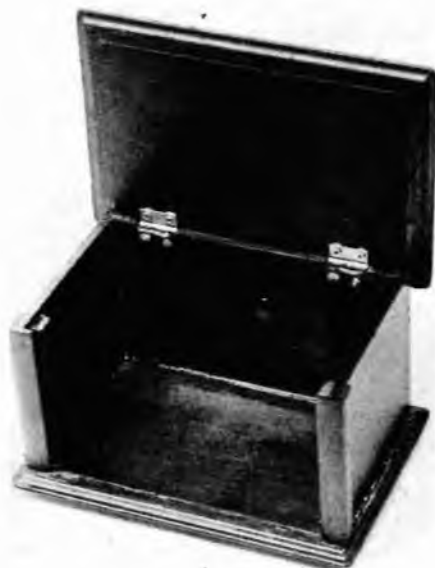
Here's the same view of the cabinet as in the drawing on the previous page. Be sure that the front panel slides in smoothly.
