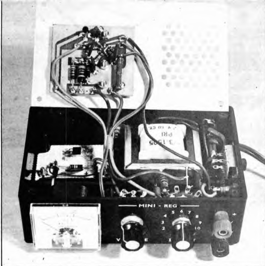
Internal view of the Mini-Reg. The circuit board is positioned so that it doesn't come in contact with the meter and transformer. The case is perforated for ventilation. You can see the tiny, square HEP 176 rectifier on the small circuit board in the bottom of the case.
