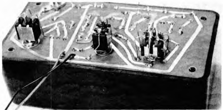
Here's the underside of the completed board with all three switches and J1 installed. The two wires leading away run to the 9-volt transistor battery which will fit in the cabinet.
