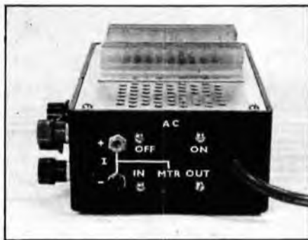
The AC line switch, current jacks and current meter switch are on the end of the case.
