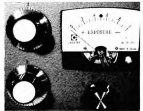
Close-up of meter face showing a small scale-illumination lamp in lower right corner. This lamp should not be operated at full voltage to avoid fogging the film.
