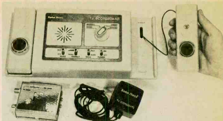
Hand-held controls extend up to nearly three feet from console, which can be as far as 12 feet from set. Front left is balun transformer, input matcher and connecting cable (right).
