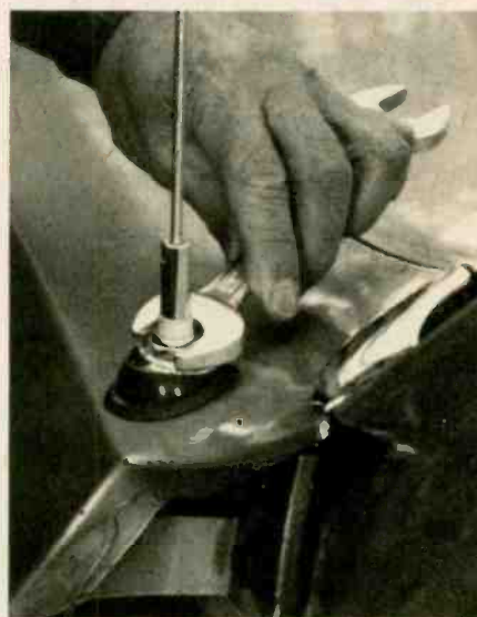
Tightening the cowl-mounted CB antenna. This location was chosen because it's easy to run lead-in cable from antenna to set.
