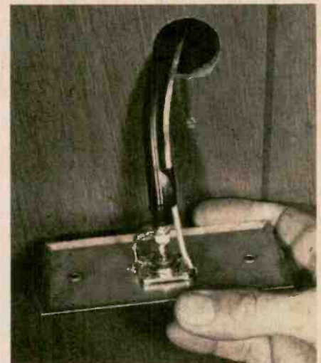
Blank electric wall socket plate was drilled to take UHF socket for high frequency coaxial cable. Single white wire on right side is separate ground.
