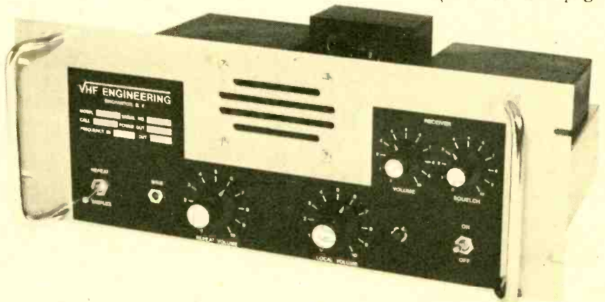
This is a repeater, the unattended, automated transmitter/receiver package that can extend the range of 2-way radio signals. This model from VHF Engineering is for use on the ham VHF band.
