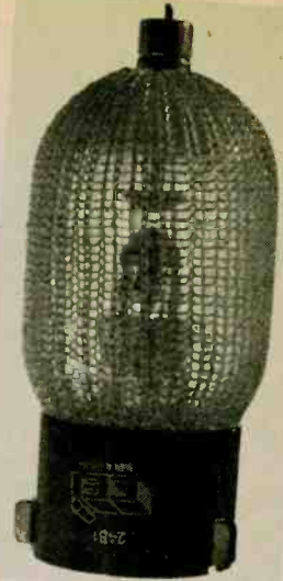
Unusual magnetron modulator used in small-craft radar has explosion-proof cover. Metal net is part of this English-made 24B1 Triggertron.
