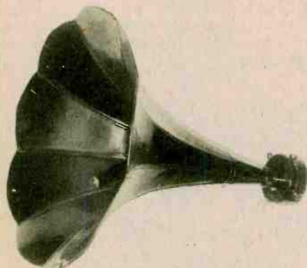
This Western Electric model 360W microphone with a 4A horn is in the collection of Lloyd Williams of Frankfort, Indiana. The microphone was originally used by telephone installers of the Western Electric and Bell Telephone companies.
