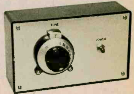
Low drain circuit is powered by three AA cells. Holder can be made from scrap piece of aluminum or bought. Vernier dial has 8 to 1 turns ratio for precise adjustment.
