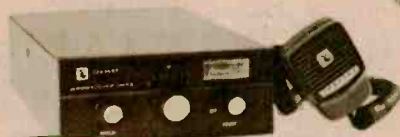
Messenger 123B 23-channel mobile with +/- ground switch
