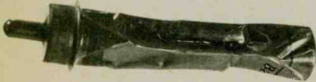
This common 1B85 geiger counter tube has a thin metal case which actually goes flat from fatigue. Atmospheric pressure on the thin metallic skin is the cause.
