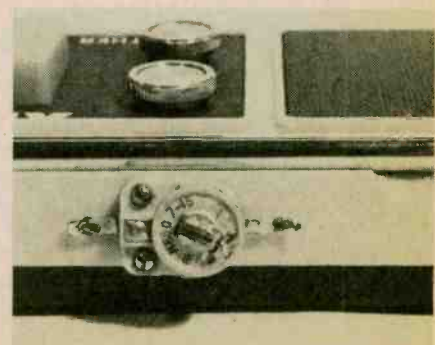
Install a small trimmer on the cabinet at a point just outside the internal trimmer.
