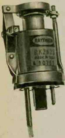
Invented in 1939 by the Varian brothers, the klystron is being replaced by step-recovery diodes as local oscillators in radar sets, although some, like this famous 2K25, are still used in police radar sets.
