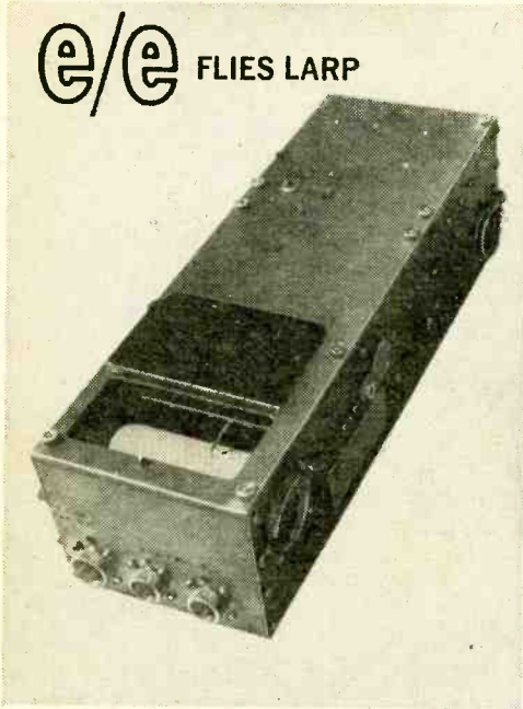
The LARP's chart recorder (left) weighs only three pounds and can record air pressure, humidity and temperature. The entire system (right) is ready for flight.
