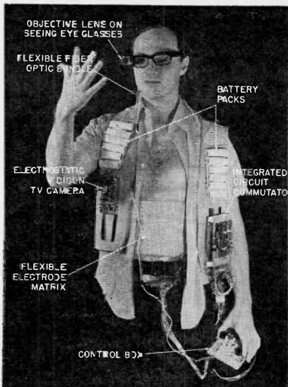
Still a bit clumsy, but toteable, the new Seeing-Eye system can be transported by a man comfortably. Here, trainee sees outline of his hand for first time.
