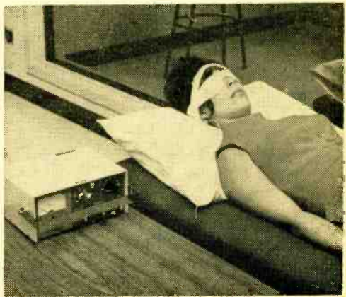
Controls for the battery-operated portable Electrosone 50 were adjusted so that the patient felt no sensation except a slight tingling. Relaxed but not actually asleep, the patient will virtually "float" until electro-sleep is ended by a preset timer.
