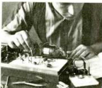
Observing transistor operating as shunt-fed amplifier — Student has installed an oscillator and shunt-fed amplifier. He takes various measurements and observes the transistor operating as an amplifier. This is a typical solid-state circuit.
