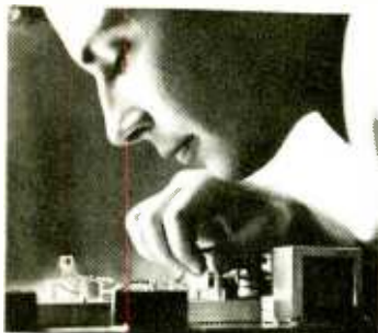
Working with basic single transistor circuit — Student learns best installation and troubleshooting techniques. He has constructed a basic single transistor circuit, first step toward understanding more complex solid-state circuitry.
