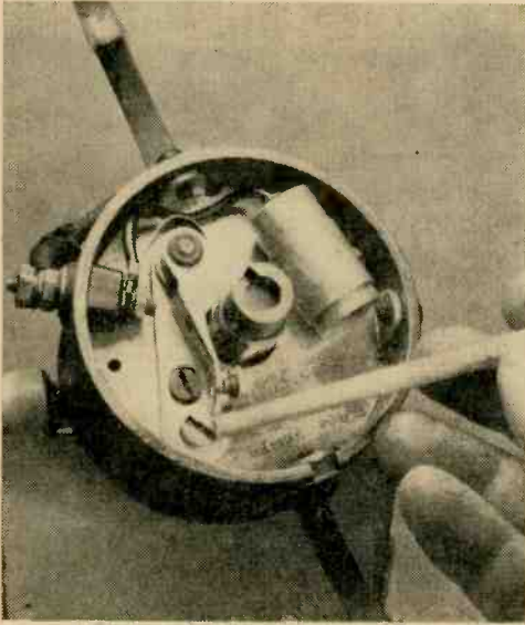
Fig. 6. The lock screw is loosened and the points are adjusted to specification. Carefully tighten screw without moving points.
