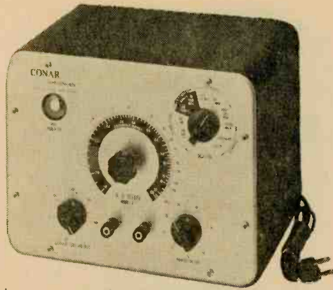
Fig. 14. Checking capacitors to determine their capacity and leakage requires a good R-C tester; also reads accurate resistance.
