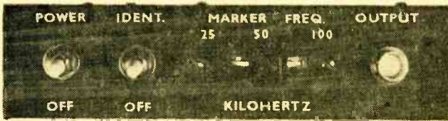
Front panel view of the Mark III details in-line arrangement for all controls. Use transfer or Datak letters for control identification to give your unit the professional appearance.
