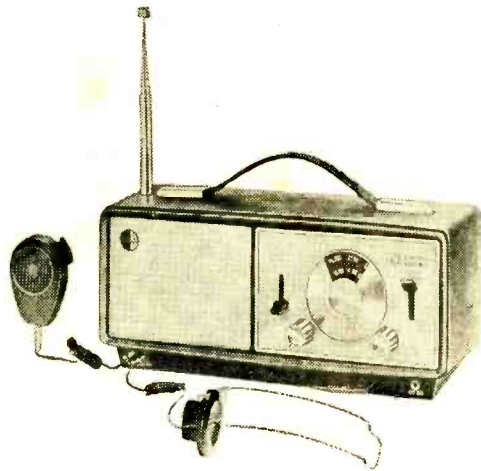
Designed especially for the Part 15 CB DXer, this little General Electric job can be used with either mike or CW key.
