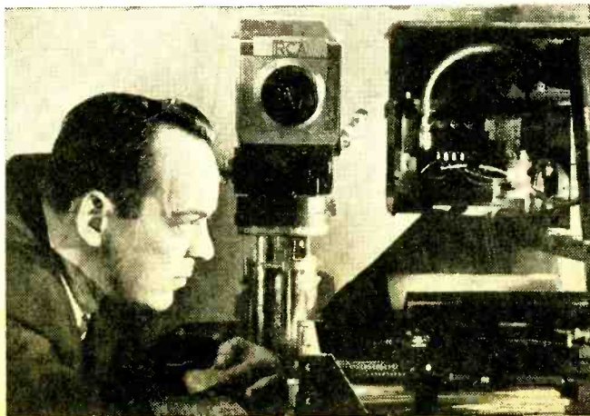
Engineer Dennis Woywood eyes RCA's new Laser Beam Image Reproducer (far right); new Return Beam Vidicon camera is in center. Though designed primarily for EROS satellite, vidicon camera could be made lightweight and compact enough for use in TIROS M advanced weather satellite, currently under construction.
