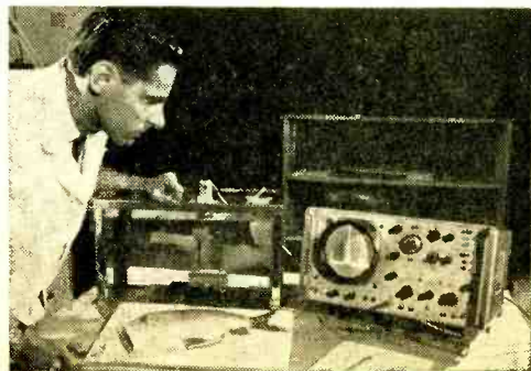
Researcher Freese using an ultra-new ultrasonic method to determine quality of frozen whitefish. Silent echo from ultrasonic sound pulse beamed at frozen fish sample is viewed on oscilloscope.
