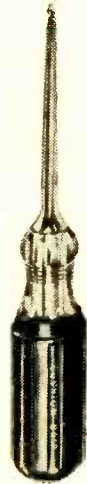
Metal nibbler (top) develops leverage through squeezing action. Cuts 18-gauge steel or aluminum. The Seizers are similar to the surgical tools that are used for clamping. Wire stripper clips on iron—cuts plastic insulation but not conductor. The Scratch awl is great for marking chassis and phenolic board and for making holes for sheetmetal screws.
