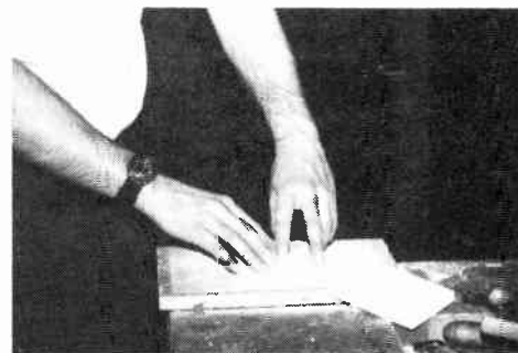
Fig. 22. Carefully sand the cut edges until they are free of saw marks.
