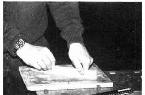
Fig. 8. Edges may be squared up on a sanding board with equal ease.
