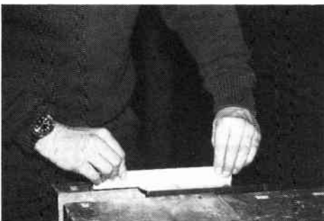
Fig. 7. Edges may be squared up using a conventional wood plane.
