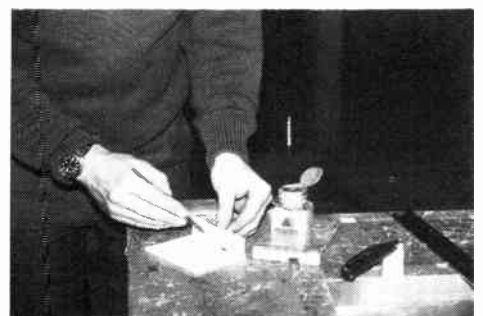
Fig. 10. Adding solvent to each side (if possible) of the joint.
