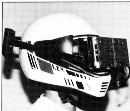
Helmet-mounted display system as used in 'virtual reality' experiments at Advanced Robotics Research Ltd.
