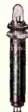
E-lite 1AD—Transistor circuit indicator light. Operates on 10-volt signal at low current. Has pre-aged neon lamp, built-in diode-resistor network.
