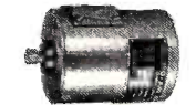
SA-526-A 115 V, 400 CPS, 1 \phi Actuator Motor, Int. duty \frac{1}{2} HP, 6 pole, 2 \frac{1}{2} " dia. x 3 \frac{1}{8} " long
