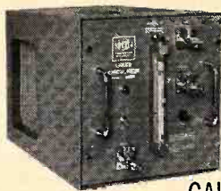
CALORIMETRIC WATTMETER LIQUID CIRCULATOR
