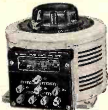
TYPE LW136 (and LW136-3) Double wound assembly with isolated secondary. One phase 120 or 240 volt input. Three uses: (1) One phase 120 or 240 volt input; 3-phase 240 or 480 volt input; low voltage isolated output. (2) 120 or 240 volt 1-phase, or 240 or 480 volt 3-phase line corrector. (3) 120 or 240 volt, 1-phase, or 240 or 480 volt, 3-phase limited range "buck-boost" variable transformer.
