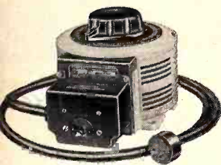
TYPE 2PF136 INPUT: 120 volts, 50/60 cycle, 1 phase. OUTPUT: 0-120/140 volts, 20.0 amperes, 2.8 KVA. With Cord-Plug, Fuse, Receptacle.
