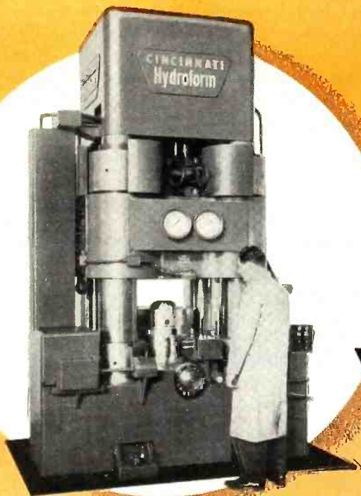
9-INCH HYDROFORM Maximum Blank 19" Diameter Maximum Draw Depth — 8"
