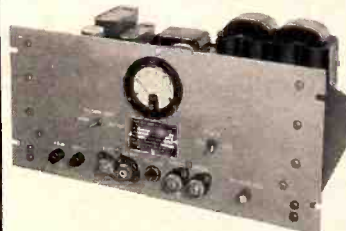
TYPE IE20003 INPUT: 95-135 volts, 60 cycle \pm 10\% , 1 phase. OUTPUT: 115 volts, 8.5 amperes, 1.0 KVA. Completely Electronic for Military Applications.
