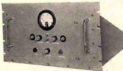
TYPE EM10009 INPUT: 187-229 volts, 3 phase, 400 cycle. OUTPUT: 208 volts, 5.0 KVA.
