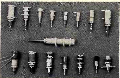
CERAMIC AND PHENOLIC COIL FORMS AND COMPLETED COILS ON SAME
