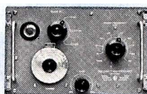
-hp- 525A Frequency Converter 10 cps to 100 MC
