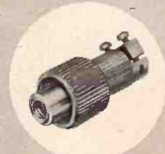
GHR Series—Approved at 2000° for 5 min. per.; hood and cable clamp protects against vibration; for No. 16 AWG; contacts 1, 2, 3, 5.
