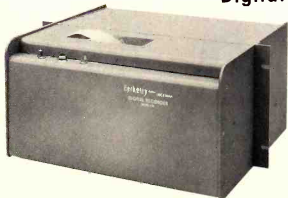
MODEL 1452 DIGITAL PRINTER. Automatically and permanently records information from any Berkeley 5510, 5571 or 7000 Series instrument, prints data in digital form on standard adding machine tape from printer and scanner in one compact unit. May be modified to print "Time" or "Code" information simultaneously with data. Rack or bench mounted; available in up to 8 digits. One printout every 0.85 seconds. Price (6-digit), $950.00.
