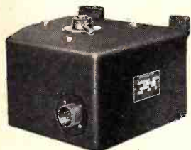
TYPE 1126-1001 INPUT: 115 volts, 400/800 cycle, 1 phase. OUTPUT: 0-130 volts, 15 amperes, 1.95 KVA. With a Dust-Proof Container.
