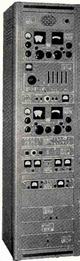
TYPICAL RECEIVER TERMINAL for TWINPLEX OPERATION
