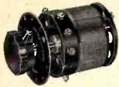
TYPE 20 INPUT: 120 volts, 60 cycle, 1 phase. OUTPUT: 0-120/140 volts, 3.0 amperes, .42 KVA for Back-of-Panel.
