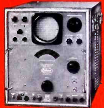
DIRECT READING SPECTRUM ANALYZER Model TSA Bandwidth 10 to 44,000 mc 5 Interchangeable Tuning Units
