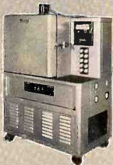
Portable 4 cu. ft. Test Chamber, range +250° F. to -100° F.
