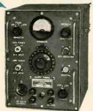
Type 560 PRECISION FREQUENCY METER 2.40-3.40 kmc/s
