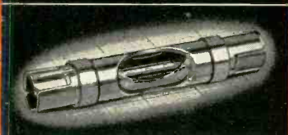
874-LR RADIATING LINE — $12.00. Short coaxial line with hole in outer conductor that can be partially or completely covered by a rotatable sleeve — for coupling to external wavemeter or heterodyne frequency meter
