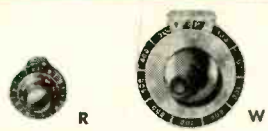
MODELS R AND W DUODIALS Each model available in standard turns-ratios of 10, 15, 25 and 40 to 1. Inner scale indicates angular position of HELIPOT sliding contact, and outer scale the helical turn on which it is located. Can be driven from knob or shaft end. R—2" diameter, exclusive of index. W—4-3/4" diameter, exclusive of index. Features finger hole in knob to speed rotation.
