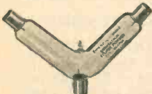
Y-Type Position Convectron—Vertical Sensing Tube.
