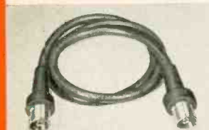
874-R20 PATCH CORD — $8.00. Three feet of Type 874-A2 Polyethylene Cable with a Type 874-C Connector on each end 874-A2 POLYETHYLENE CABLE — $0.50/ft., $27.00/100 ft. Bulk cable — characteristic impedance of 50 ohms \pm 5\% — double-shielded — good mechanical flexibility
