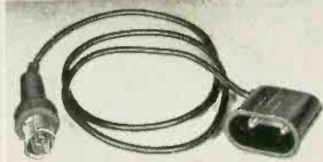
874-R31 PATCH CORD — $4.50. Three-foot, flexible coaxial cable terminated with Type 874 Connector and phone tips
