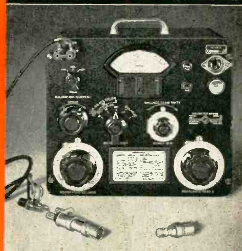
1651-A BOLOMETER BRIDGE. For conveniently measuring h-f power by either d-c substitution or direct-reading method with the following three bolometer units:
