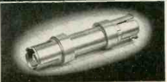
874-K COUPLING CAPACITOR — $12.00 Short coaxial line with 0.005 microfarad capacitor in series with inner conductor — transmits h.f., blocks d.c.
