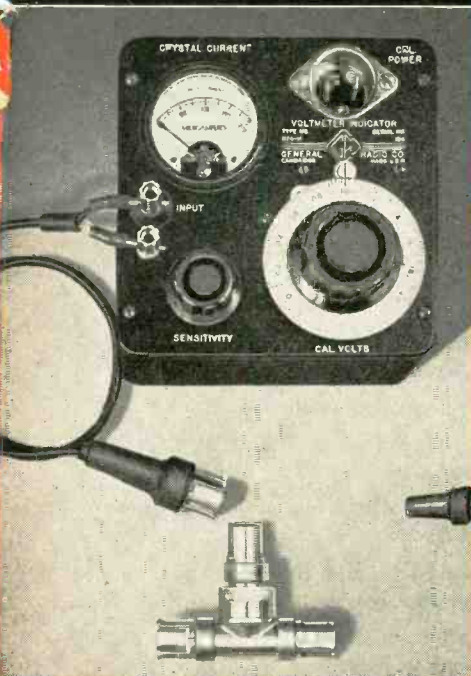
874-VR VOLTMETER RECTIFIER — $25.00. Crystal rectifier across short coaxial line — useful frequency range 15 Mc to 2,500 Mc — resistor in series with inner conductor provides 50-ohm source impedance — also useful as detector (illustrated at bottom)
