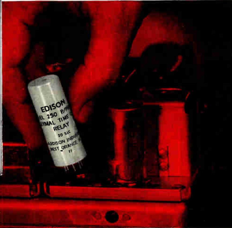
Edison's Thermal Time Delay Relay being inserted in the CAX-12 servo power unit.
