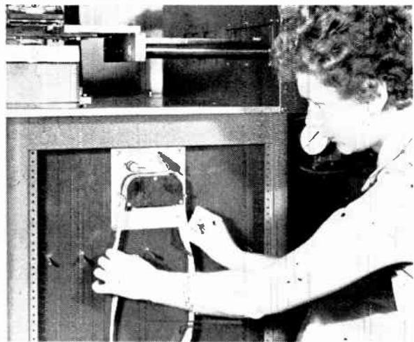
Operator inserts tape to run Design Tool's assembly machine
