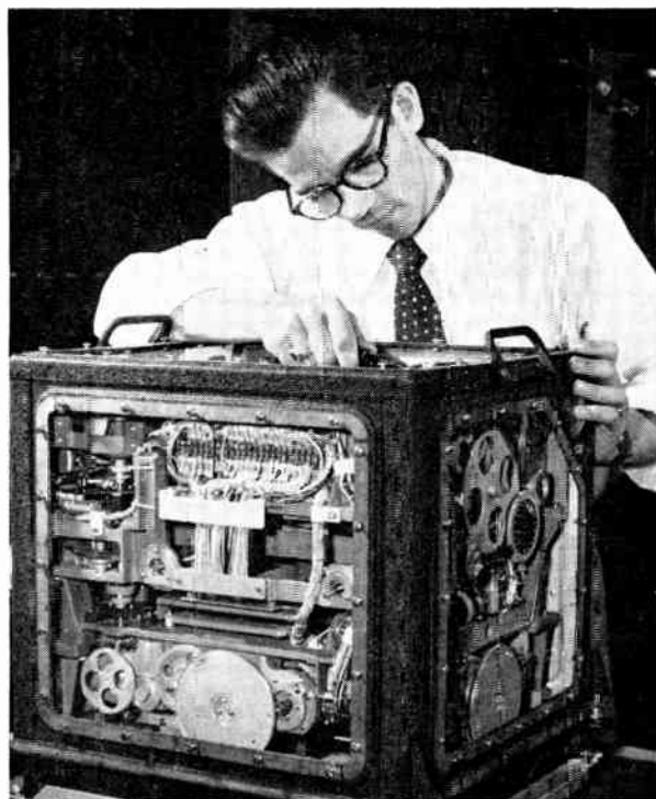
K-system bombing/navigational computer used in B-47 medium bombers and early B-52 heavy bombers
