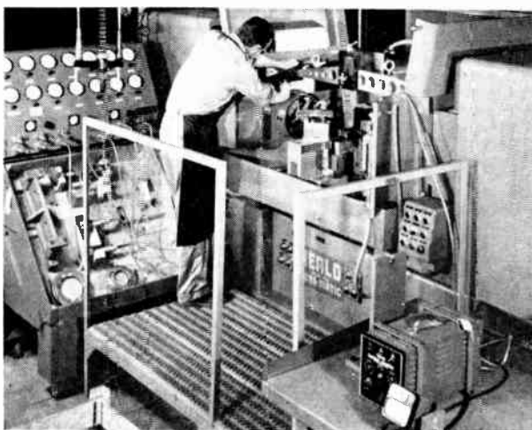
Gyro gimbals for guided missile are machined to ultra-close tolerances measured in millionths of one in. Electronic bridge gage (center) checks flatness, squareness
