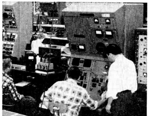
Flight test equipment for inertial-guidance systems. Frequency standard includes a master electronic clock. It is accurate to one second per day
