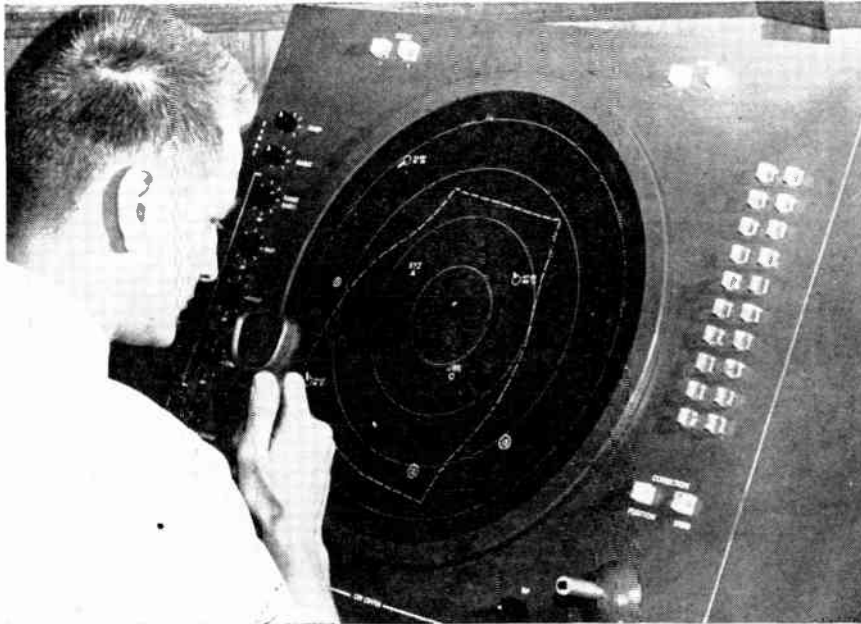
Symbols can be superimposed on radar presentation to aid flight controllers at busy air terminals
