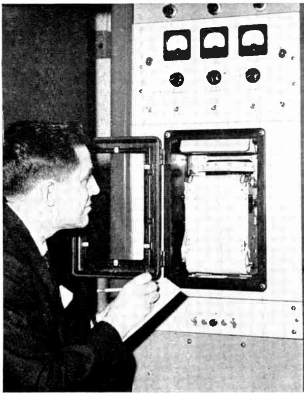
Monitor strip chart gives dosimetry record. Monitor computes beam current, beam energy and scanning current, sounds alarm on variation of 5 percent
