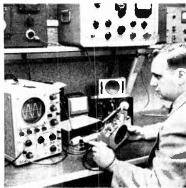
Engineer checks 4-transistor reflex receiver for distortion
