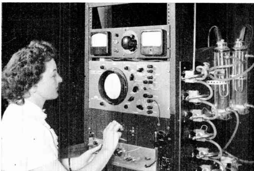
Thermal resistance measurement equipment, another Clevite development, is used to check temperature drop between the junction and mounting base of power transistors under actual operating conditions. It's one of many specialized testing procedures to control quality and improve performance.
