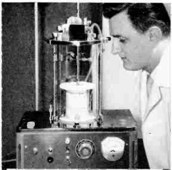
Continuous vertical crystal puller, developed by Clevite engineers, has tremendously improved the crystal-growing art. It is just one indication of the solid-state knowledge and volume production set up that keeps Clevite in the forefront of semiconductor developments.
