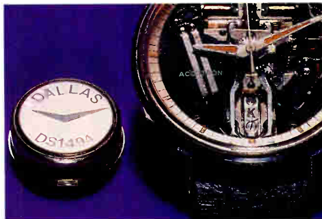
Dallas Semiconductor's Time-in-a-Can offers a full-feature full-time clock in the industry's smallest package.
