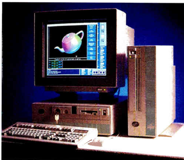
The RS/6000 model 320 desktop workstation now renders 3-d graphics at a rate of almost 1 million vectors/s.
