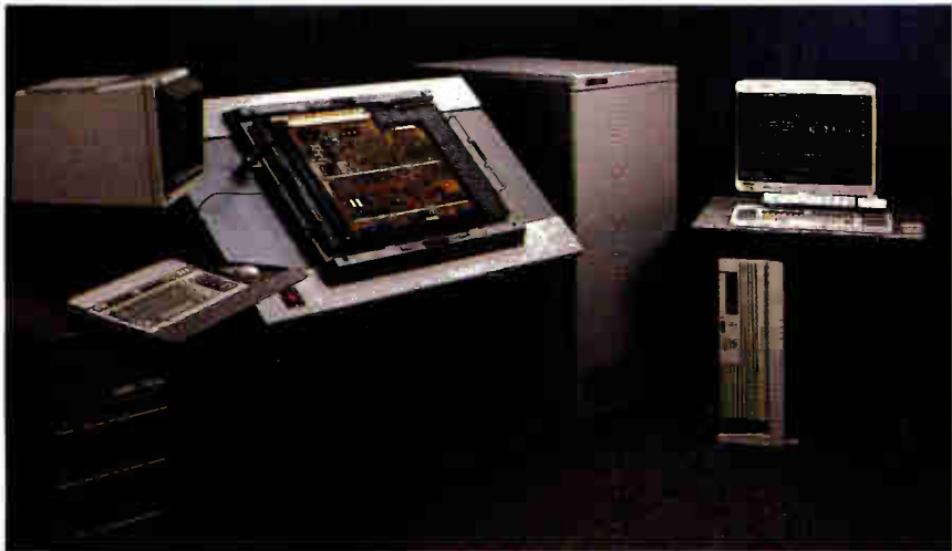
Schlumberger's S780 board-test system comes with a computer-aided test-engineering workstation to run its software.
