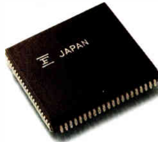
1.5 \mu 3000 Gate CMOS Gate Array
