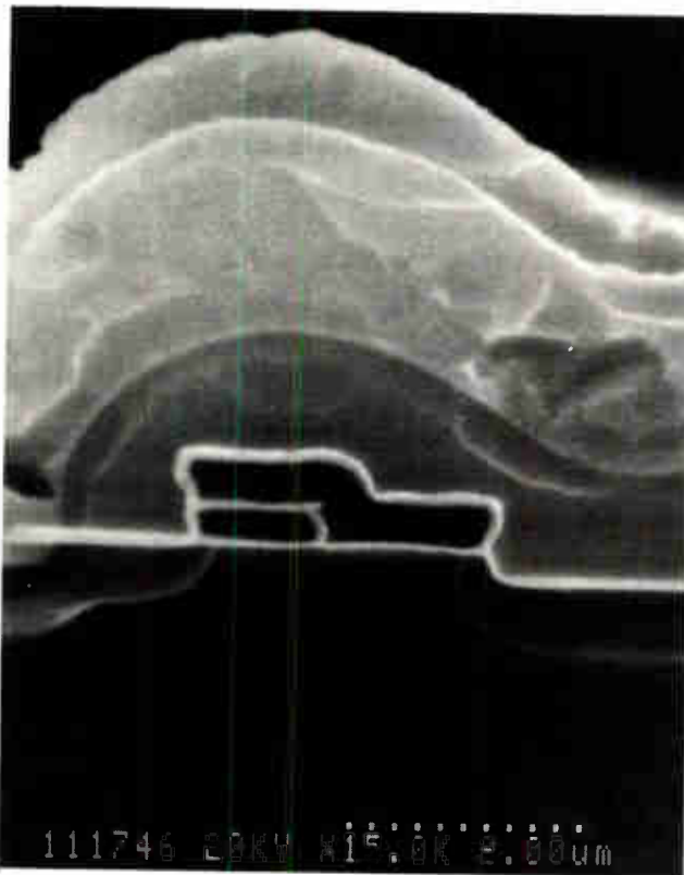
In Seeq's design, a control gate overlapping the floating gate creates a phantom select transistor, so no external transistor is needed.
