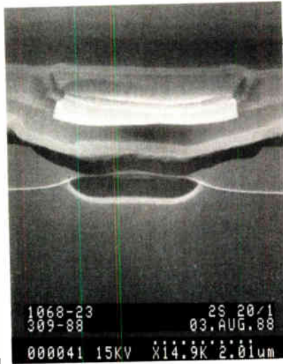
Actel uses antifuse technology in one-time-programmable gate arrays.
