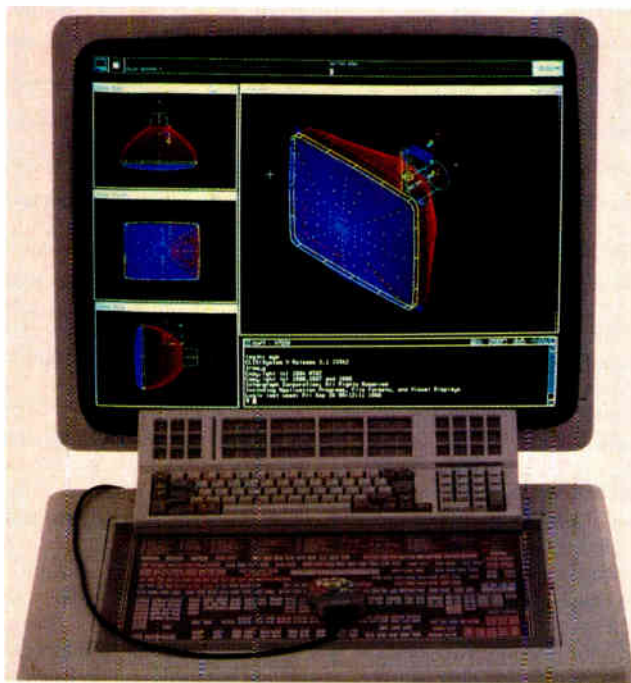
A screen measuring 27 in. on the diagonal, which displays 1,664 by 1,248 pixels, is available on Intergraph's model 3070 work station.
