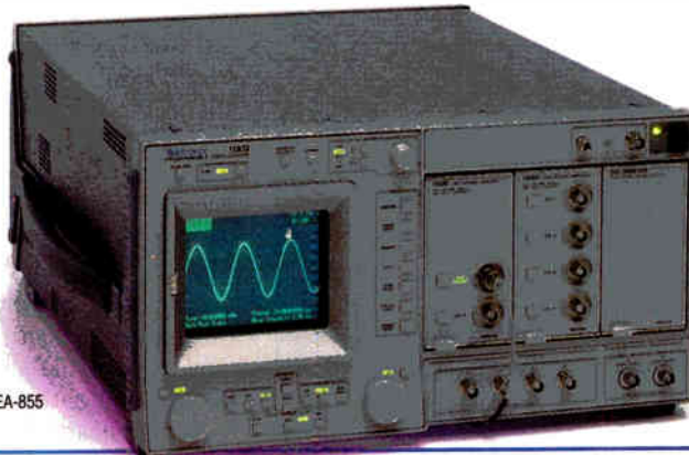
Make gated pulse width measurements with counter accuracy. Center is counterview trace, bottom clearly shows pulse width measured.
