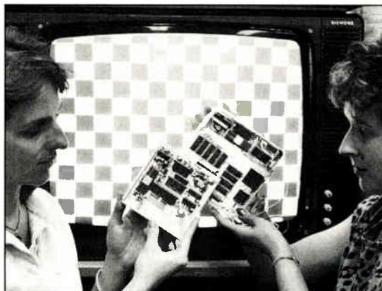
Cards from Philips and Siemens digitize TV color signal processing and horizontal and vertical deflection.
