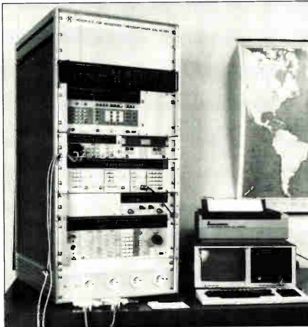
WIDE RANGE. The TS9020 calibrates and adjusts signal generators and test receivers operating at audio through radio frequencies.
