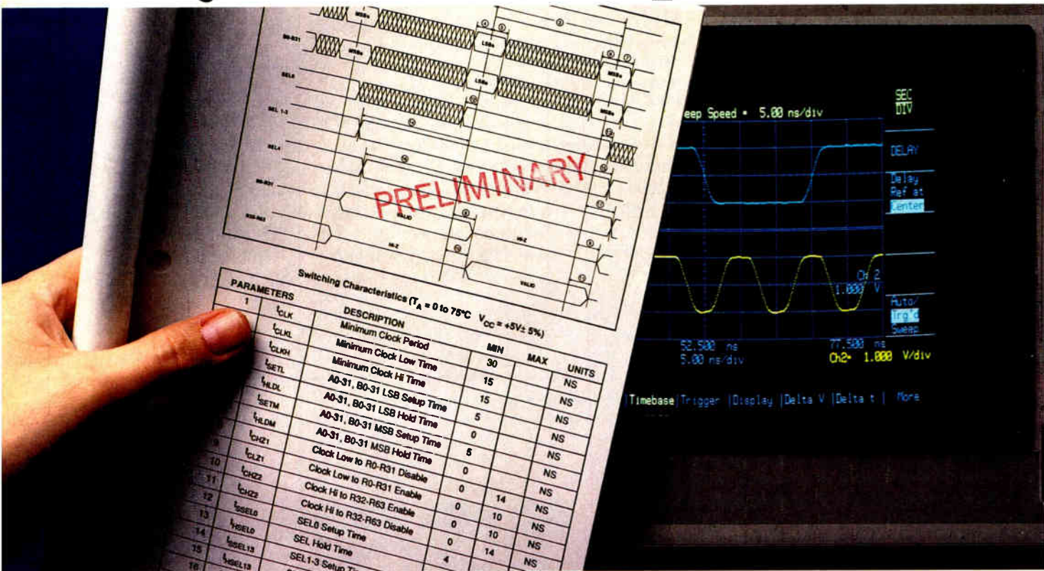
Teradyne J953 VLSI test system waveforms observed with a 1GHz digitizing oscilloscope.
