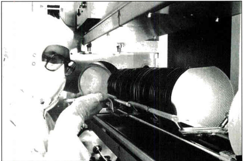
ON THE LINE. Performance Semiconductor uses 6-in. wafers on this fab line for its 12-ns, 64-Kbit SRAMs. The company finds testing the parts more difficult than using them.
