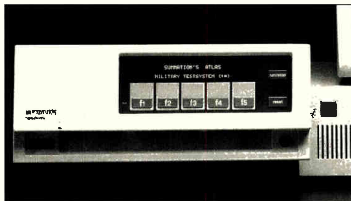
1. SMART TEST STATION. A microprocessor in the test station (left) executes test programs downloaded by a personal computer (right).
