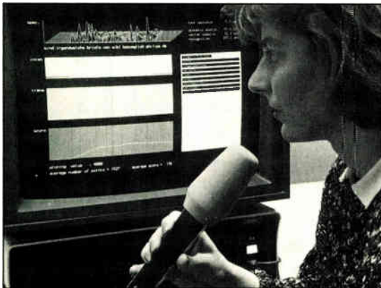
TALKATIVE. The Spicos dialog system understands fluent, continuous speech and replies to the speaker.
