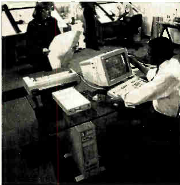
HIGH END. Model 80, shown with a 16-in. display and an external 5¼-in. floppy-disk drive, tops IBM's Personal System/2 line.
