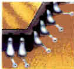
With a better matched CTE, PC boards of COR-LAM prevent solder joint cracking.
