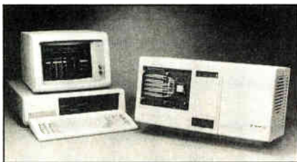
SMART. Logic Master ST uses an IBM Corp. PC XT as its controller.
