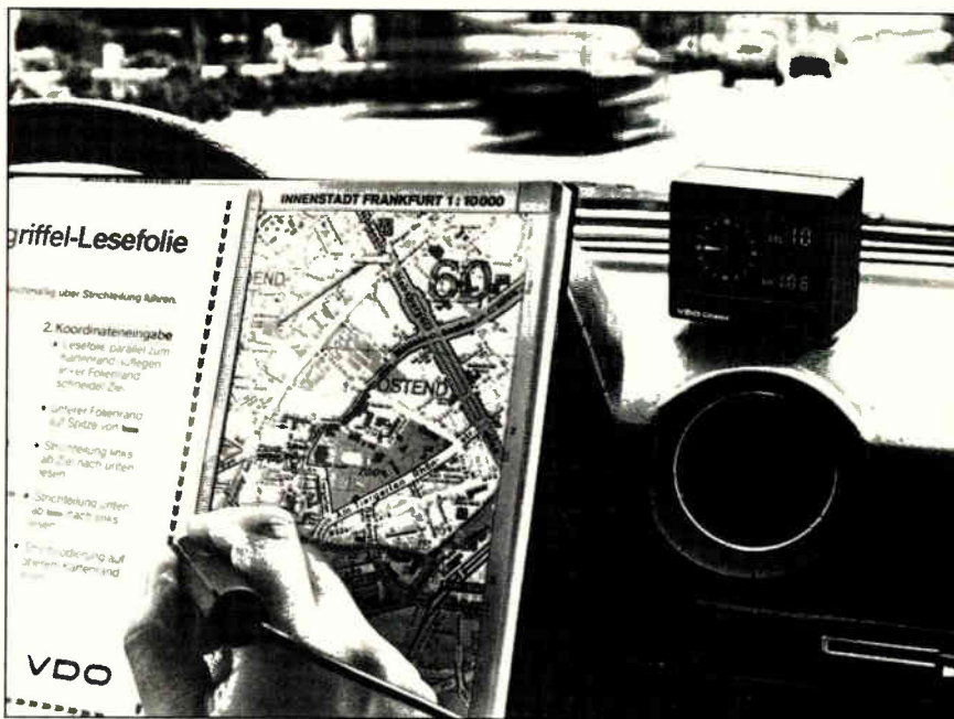
RAMBLING WAYS. Data for a journey is picked up from a bar-coded map by light pen and fed into Citypilot's microcomputer. Distance and location information is displayed on an LCD.
